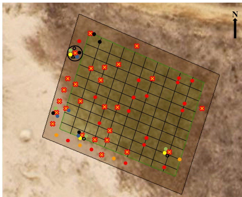
Figure 3-6. Plot #1 detections in soil for the May 26-27, 2009 sampling analyzed with HPLC. The region shaded is green is the planted portion. The fringe around the edge is unplanted (12 ft wide).
